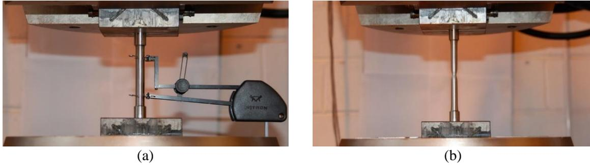
Figure 7: Coupon test setup: (a) extensometer with 50 mm gauge length; and (b) necking
