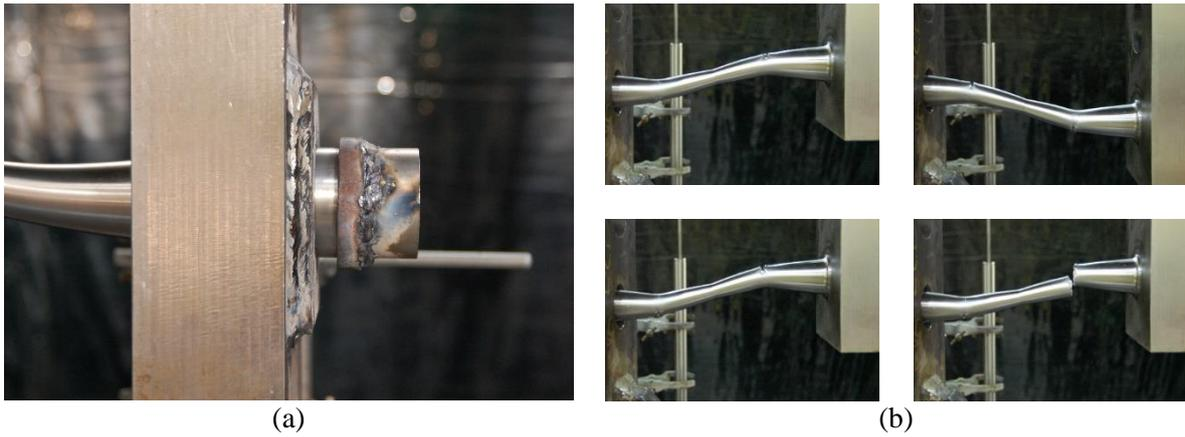
Figure 18: SSD-WHP2 (CA test at  $4u_y$ ): (a) axial expansion; and (b) final cycle with full fracture
