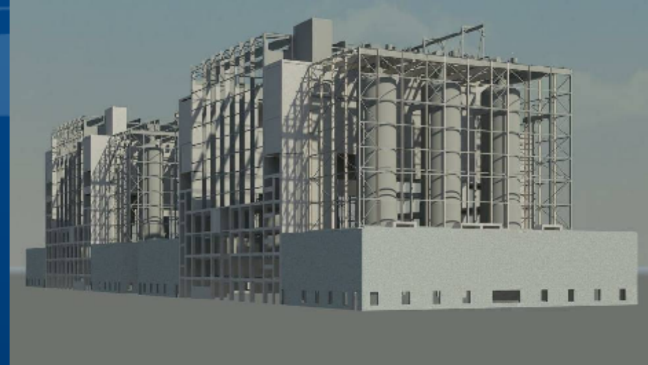
3D model of existing external envelope taken directly from the 3d laser scan 'point cloud' data
