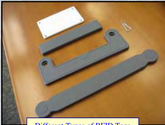
Different Types of RFID Tags
