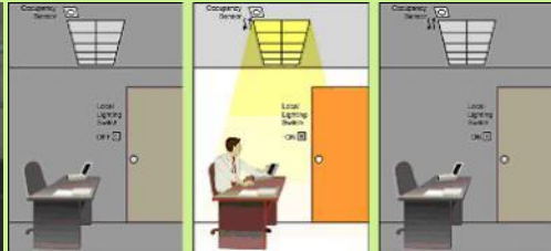
On/off control of fan coil units in each classroom is interlocked with lighting
