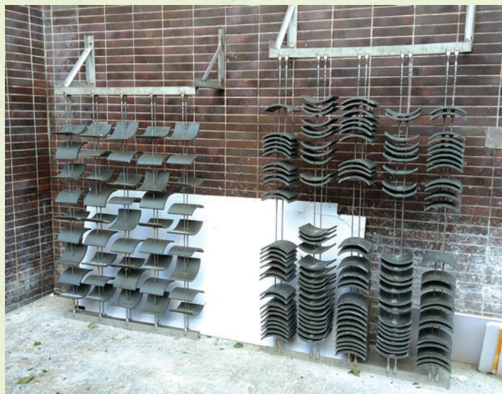
Mock-up test for the proposed façade wall.
