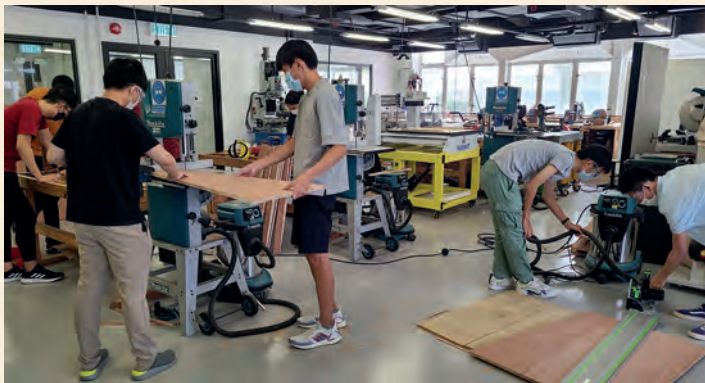
Students participated in a workshop to construct wooden molds for the bench supporting structures.
