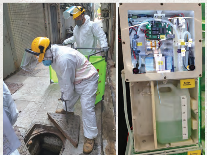
Left: The workers install the In-manhole sampling robot for sample collection. Right: The prototype of the In-manhole sampling robot.
