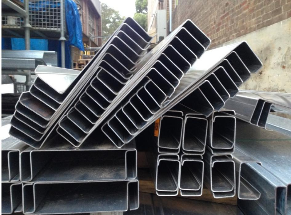
Figure 1: Cold-rolled C- and Z- sections
