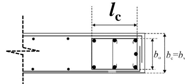
Figure above shows the confined core area reduction factor  $\alpha_n$
