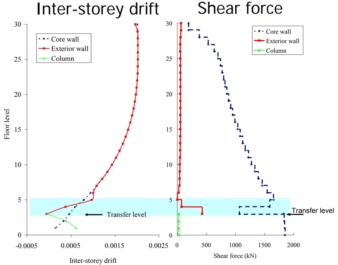
The difference in wall rotations above the transfer structure causes shear concentration in walls.
