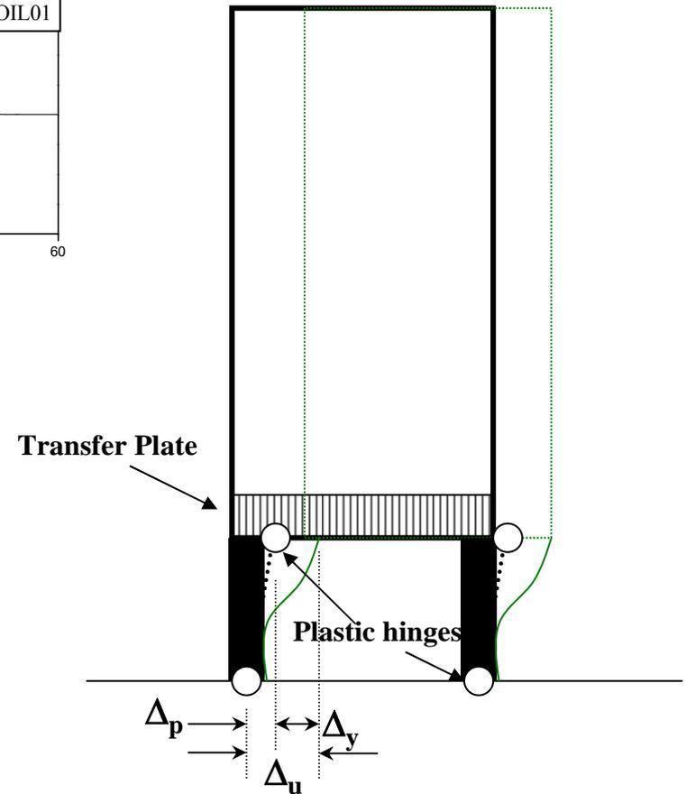
Potential Soft-Storey Failure Mechanism
