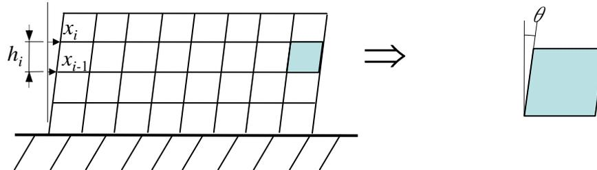
Sway deformation of frame under lateral load
