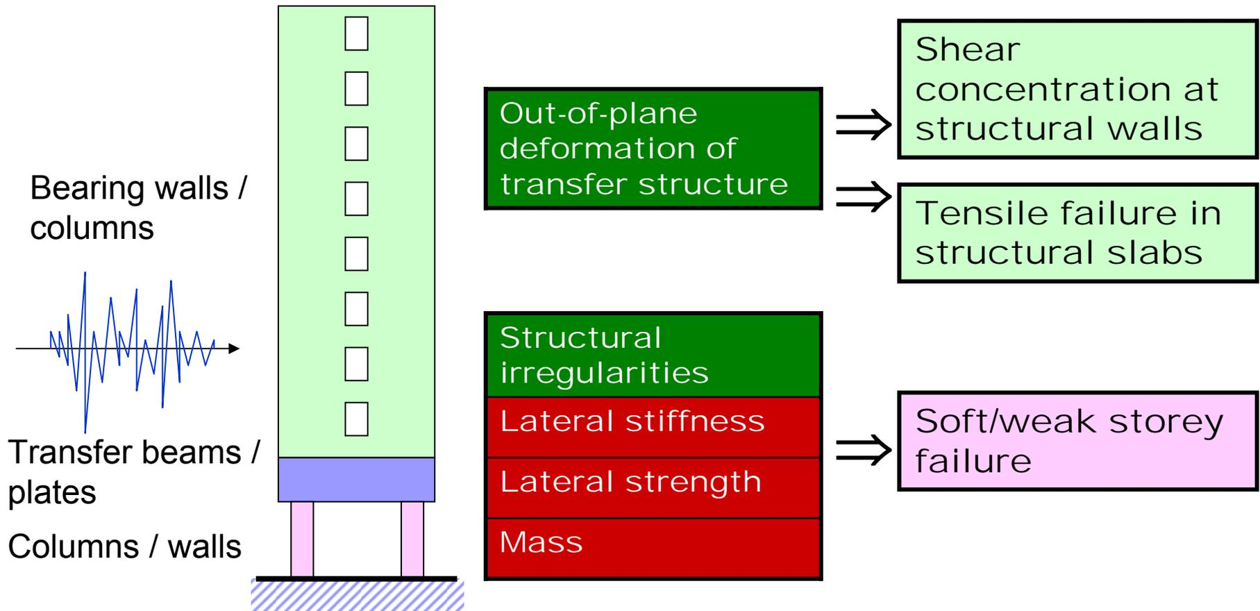
Those failure modes will be examined under the HK design based earthquake (DBE) loads.
