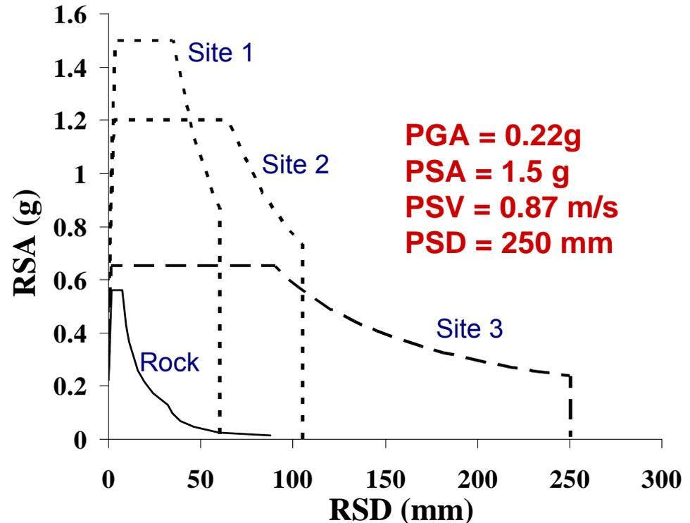
Seismic response is significantly affected by the type of sites and RP considered. Rock sites are better as their seismic response is the lowest.
