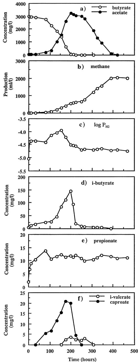
Fig. 1. Concentrations of by-products in batch degradation of  $3000 \text{ mg l}^{-1}$  of butyrate: (a) butyrate and acetate, (b) methane production, (c)  $P_{\text{H}_2}$ , (d) *i*-butyrate, (e) propionate, and (f) *i*-valerate and caproate.
