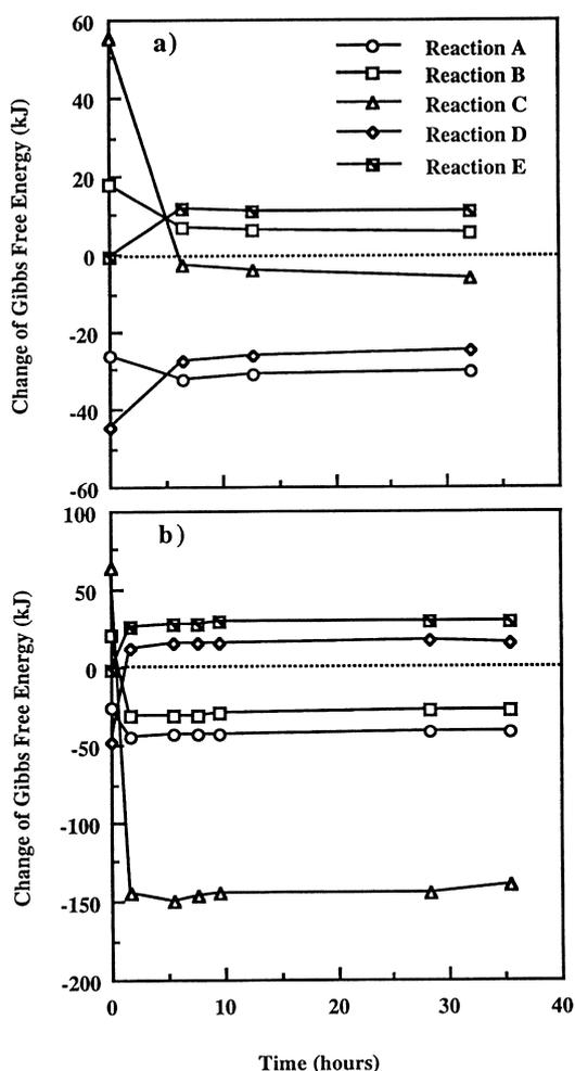
Fig. 4. Changes of standard Gibbs free energy in propionate-forming reactions in experiments using: (a) butyrate as sole substrate, and (b) butyrate and formate as co-substrate.
