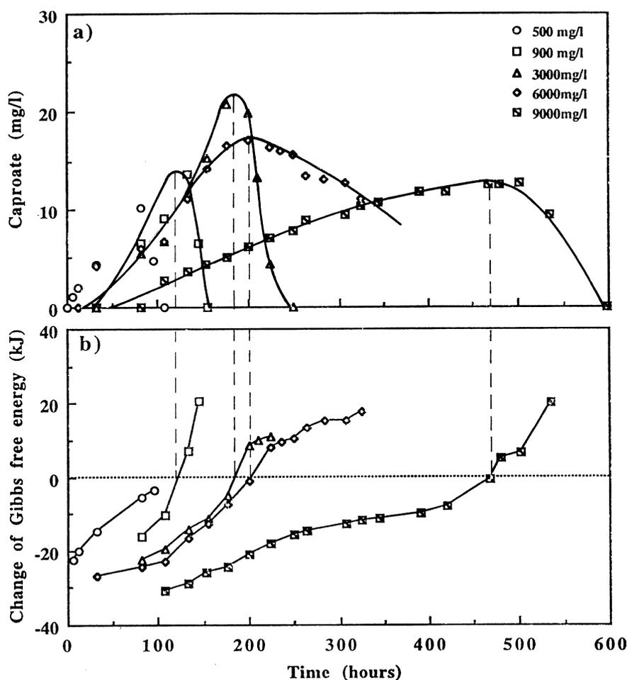
Fig. 5. Changes of (a) caproate concentration, and (b)  $\Delta G$  for reaction (F) converting butyrate to caproate.
