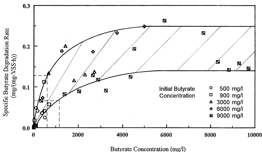
Fig. 2. Specific butyrate degradation rate at various concentrations.
