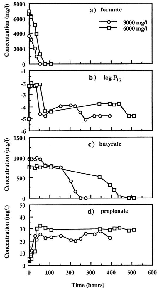
Fig. 3. Concentrations of reactants and products during the degradation of butyrate using formate as co-substrate: (a) formate, (b)  $P_{H_2}$ , (c) butyrate, and (d) propionate.
