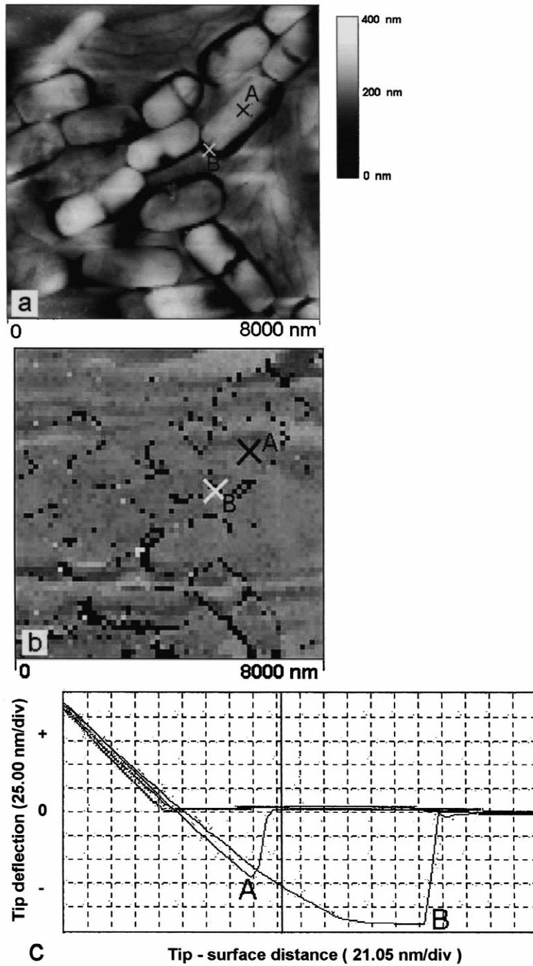
Fig. 4. (a) Contact mode AFM image of a developing biofilm, (b) the corresponding force distribution map, and (c) force curves at locations A and B.
