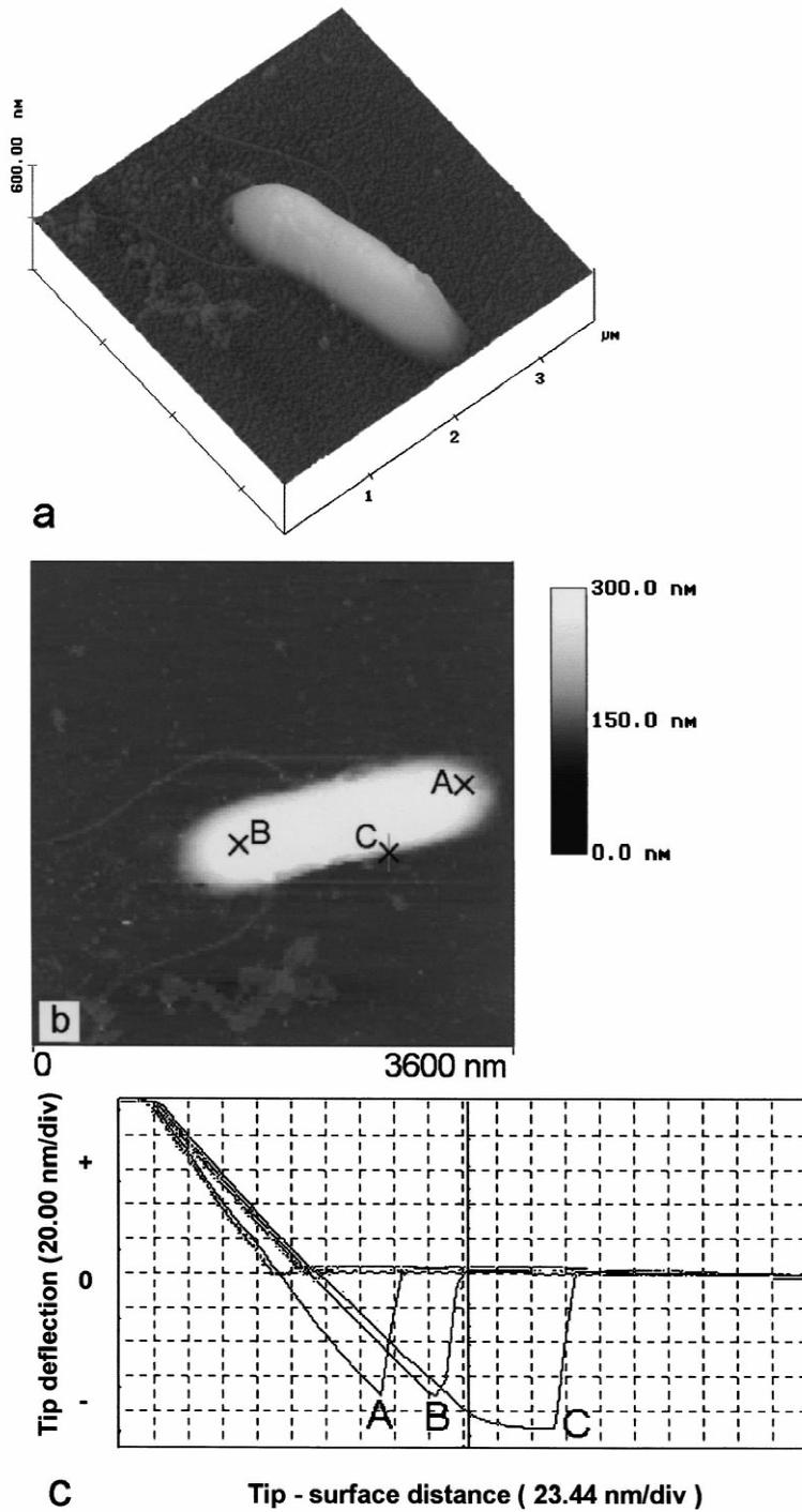
Fig. 3. Contact mode AFM images of a bacterial cell in (a) 3-D display, (b) 2-D display, and (c) the corresponding force curves at locations A, B, and C.
