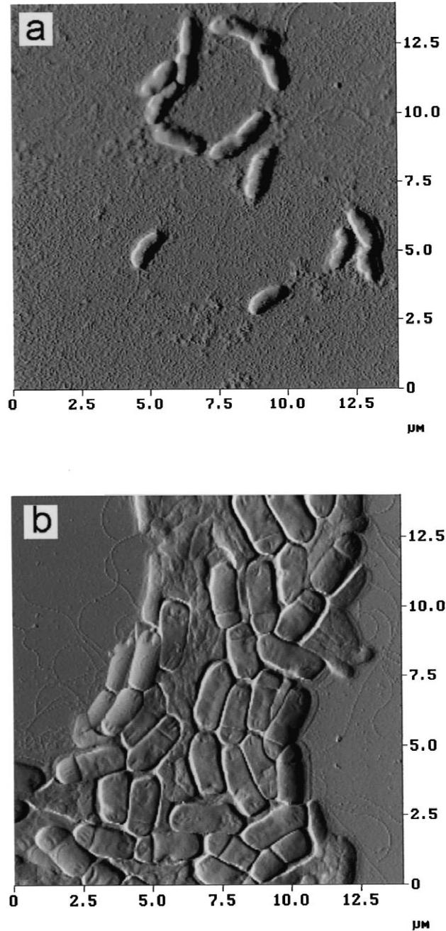
Fig. 1. Contact mode AFM images of a mica surface with (a) scattered SRB cells and (b) clustered SRB cells.
