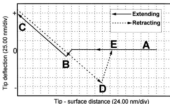
Fig. 2. A typical force–distance curve between the AFM tip and bacterium surface.
