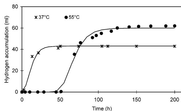
Fig. 1. Cumulative hydrogen production from starch at thermophilic and mesophilic conditions.
