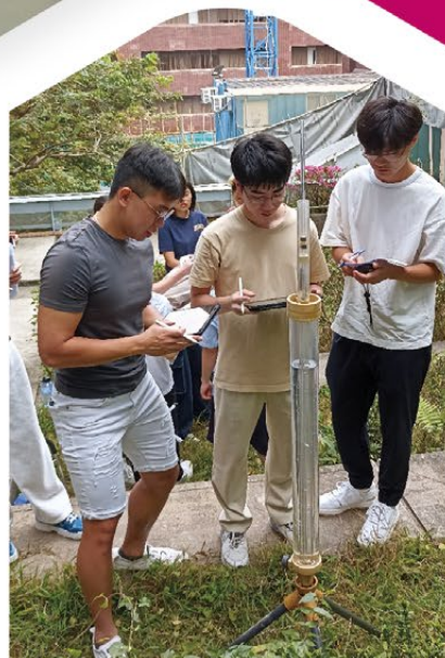
« Students visiting a foundation construction site in Hong Kong » Fieldwork measurement of soil permeability »
